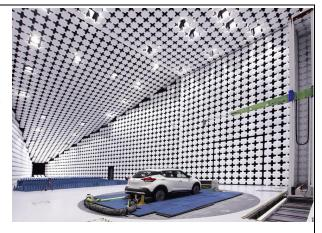
system that could have a profound impact on safety, reliability, and performance. The importance of OTA propagation for the sensors essential for ADAS operation has intensified the need for measurement facilities with enhanced sensitivity, capability, and increased frequency coverage in a simulated real-world environment. A few of the more significant test techniques are presented along with a discussion on their challenges and merits.
